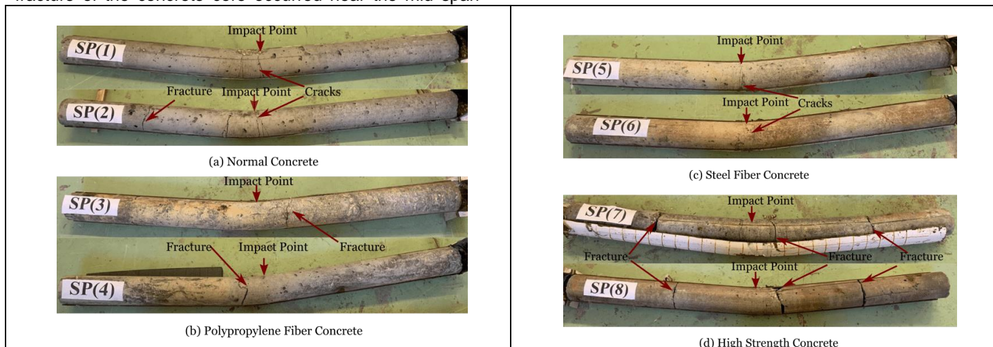
FIG. 11. FAILURE PATTERN OF THE SPECIMENS.
